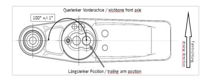
5.7.4 The position of the steering wheel on the front axle control arm in each Car is determined by spacer washers with a thickness of 8.5mm and part numbers as follows:
